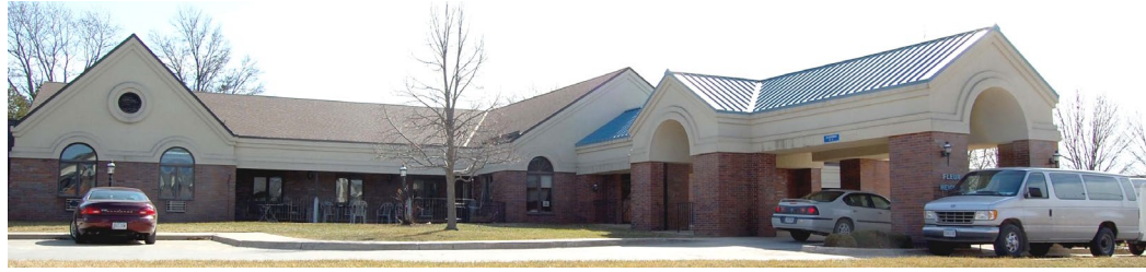
2 GRADE BRICK VENEER – WOOD FRAME
