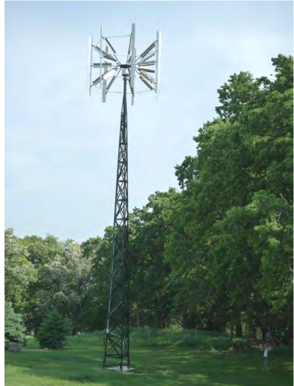
LATTICE TOWER WIND TURBINE
